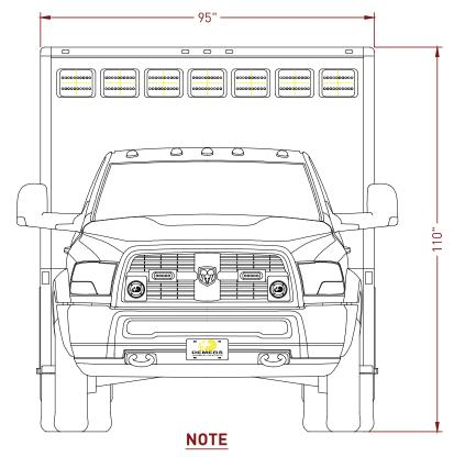
THE TOTAL HEIGHT OF THE VEHICLE CAN BE DIFFERENT ACCORDING TO CHASSIS AND SUSPENSIONS
