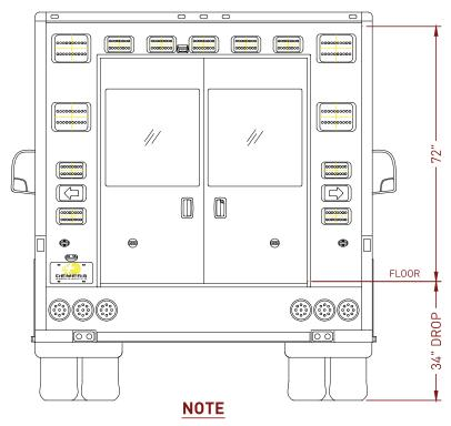
THE REAR LOADING HEIGHT OF THE VEHICLE CAN BE DIFFERENT ACCORDING TO CHASSIS AND SUSPENSIONS
