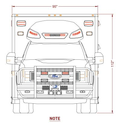
THE TOTAL HEIGHT OF THE VEHICLE CAN BE DIFFERENT ACCORDING TO CHASSIS AND SUSPENSIONS
