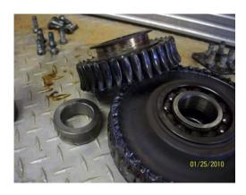
The gear case drawing shows the gears and the red line shows the oil level. If the two upper gears are spun by the movement of water through the pump, (Pump NOT IN GEAR) then this will not let the gear case lubricate the upper gears as designed. The resulting damage is seen in the picture above.
