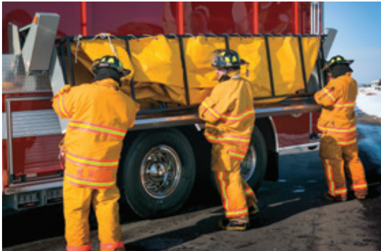
Swingdown folding tank storage. Shown on a custom dry-side tanker.
