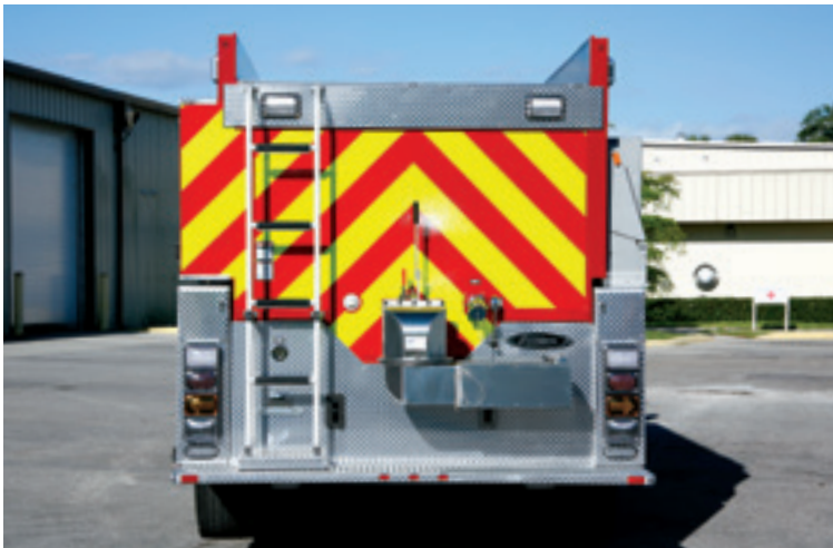
Swivel dump valve and safe access to hose bed. Shown on a BX™ tanker.
