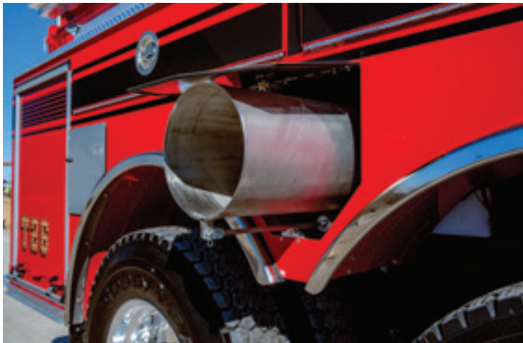
Side dump. Shown on a custom dry-side tanker.
