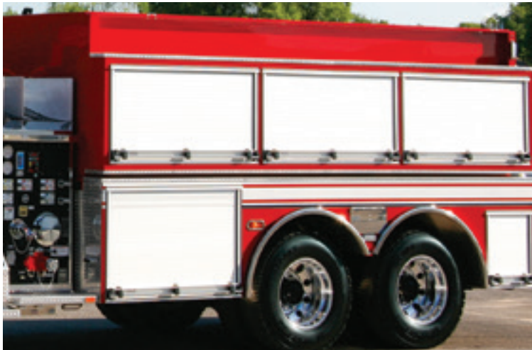
High side compartmentation. Shown on a BX™ tanker.
