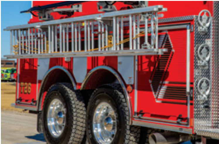
Dropdown ladder rack storage. Shown on a custom dry-side tanker.
