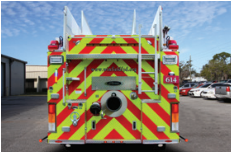
Rear dump. Shown on a commercial dry-side tanker.
